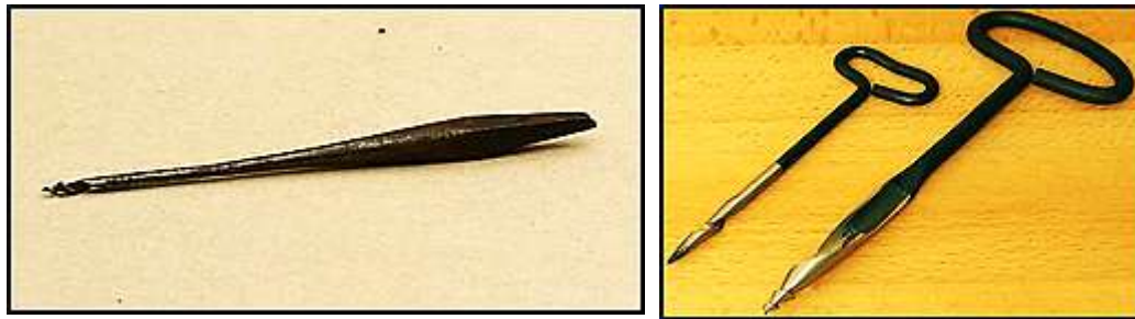
Gimlet bit for wood, made sometime before 1950.
