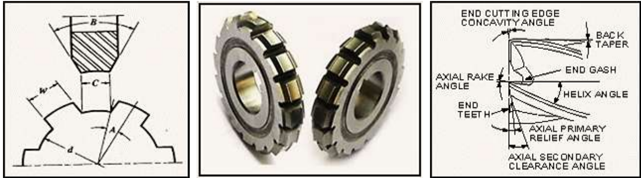
Spline shaft cutter and form milling cutter with drill flutes
