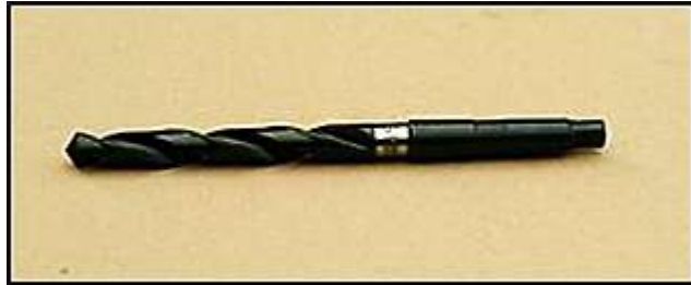
Twist drill bit with Morse taper shank and 11/32" (8 mm) drill bits - long-series Morse or plain Morse
