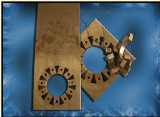
Small tooling inserts made by wire EDM
