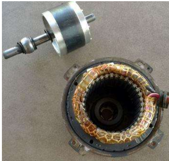
Figure 3. Electrical motor of an AC unit, including magnetic ceramics.
