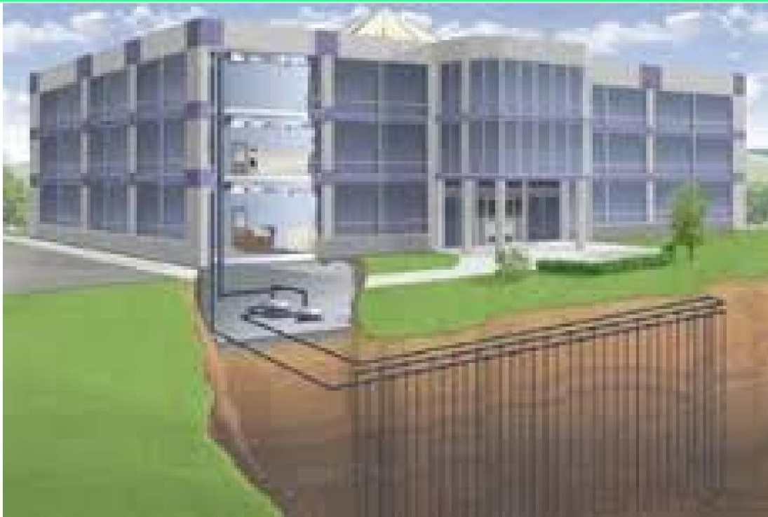
Figure 10 Deep Vertical Wells for Large Commercial structure
