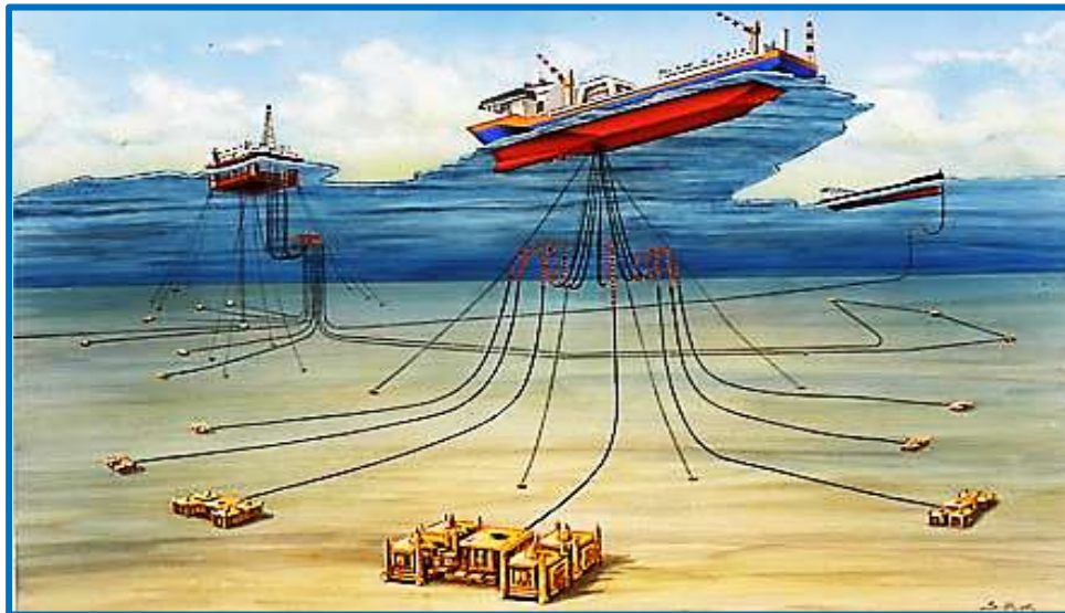
Subsea Wellheads and Christmas trees
