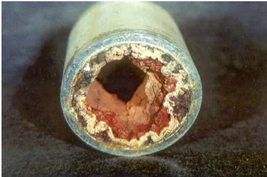
Figure 1.5 Scaled Boiler Tube
