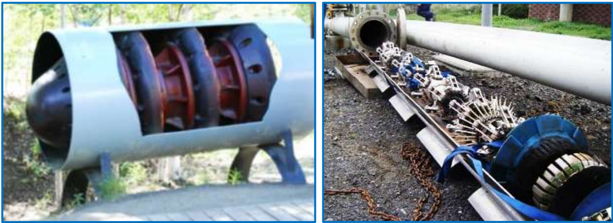
Pipeline inspection with "pigs"
