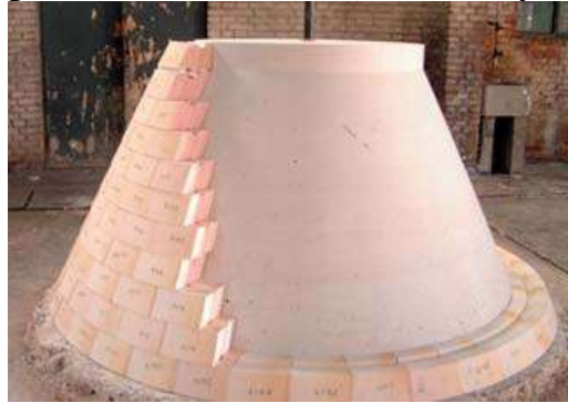
Figure 9 Monolithic refractory casted in required shape
