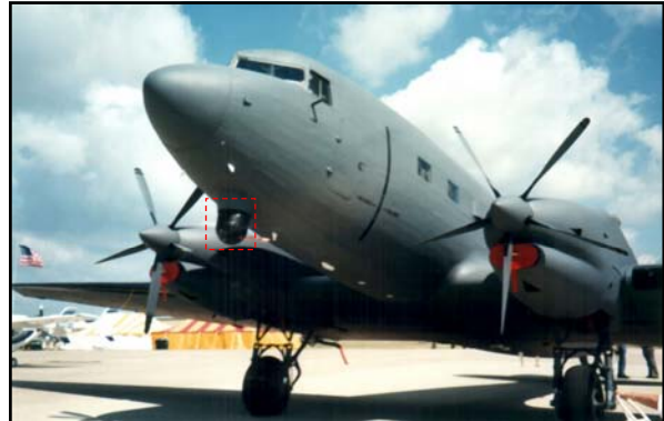
Caption: "The bubble below the nose of this BT-67 gunship is the forward looking infrared camera. All BT-67s have overwing exhausts to minimize their infrared signatures."
