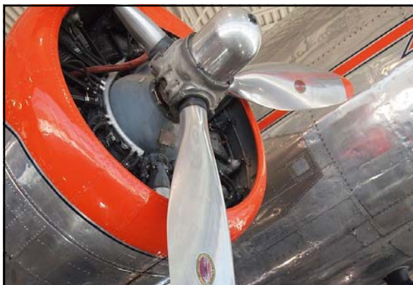
Caption: "Wright R-1820 Cyclone 9 and Hamilton Standard propeller of American Airlines Douglas DC-3"
