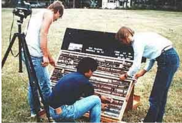
Figure 12: Handling and photographing rock cores placed in protective crates that are properly labeled in preparation for shipping and storage.
